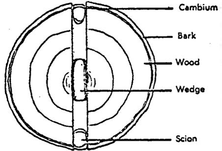
Figure 7. How the wedge is placed in the split.
